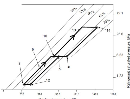
Figure 2: The cycle of the lithium bromide solution shown on the equilibrium chart.
