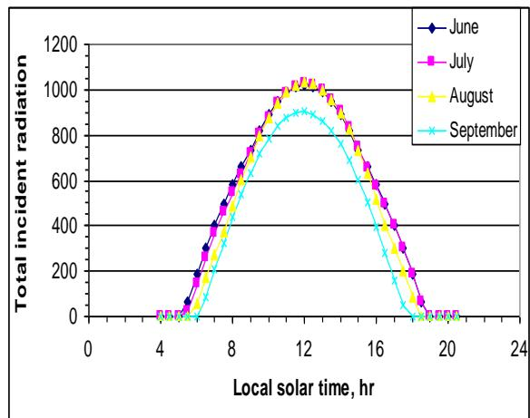
Figure 3: Total solar flux (W) computed on the 15<sup>th</sup> day for the indicated months.
